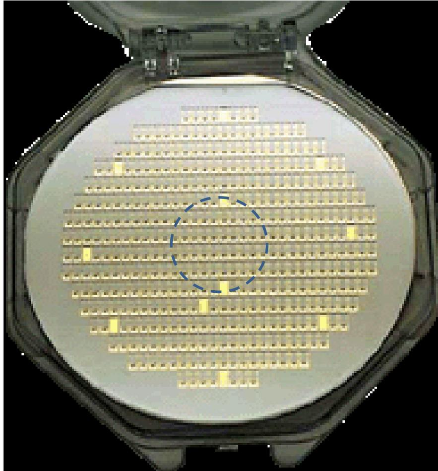
Wafer of cantilever chips
