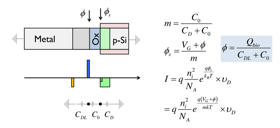
Although I have used  $\phi$  as an effective gate voltage, it should be really be viewed as a change in flat-band voltage
