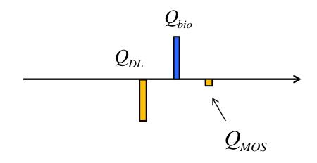
$$Q_{MOS} \approx C_{ox} \psi_{0} \propto \frac{2k_{B}T_{L}}{zq} \ln \frac{Q_{bio}}{Q_{0}}$$
