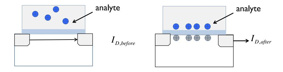
$$S \equiv \frac{I_{D,after} - I_{D,before}}{I_{D,before}} \equiv \frac{\Delta I_{D}}{I_{D}} \propto \rho_{0}$$
