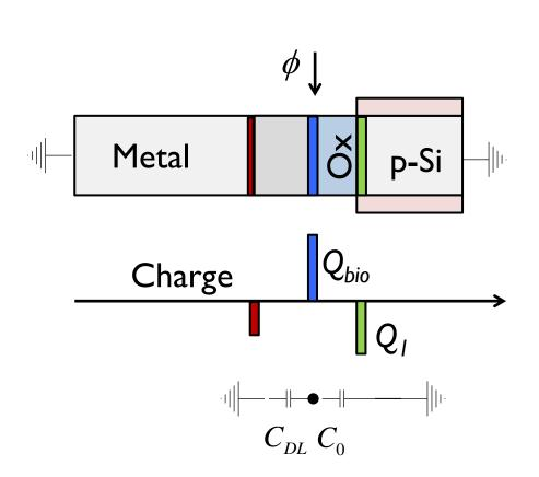
$$\phi = \frac{Q_{bio}}{C_{DL} + C_0}$$
