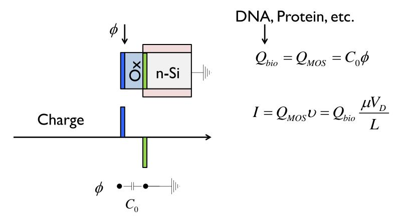
The role of charge can be viewed as shifting the flat-band voltage
