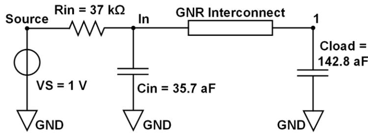
**Figure 7** Circuit for DC simulations
