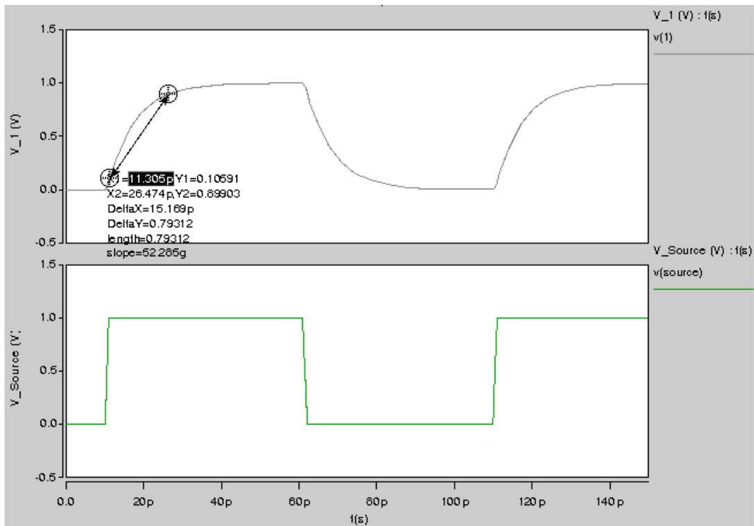
**Figure 8** Source voltage ( $V_{Source}$ ) and output voltage ( $V_1$ ). The 10%-90% rise time of the output voltage is measured as 15 ps.
