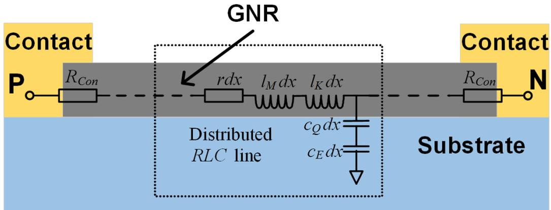
**Figure 1** Schematic of a GNR interconnect and corresponding RLC distributed circuit model
