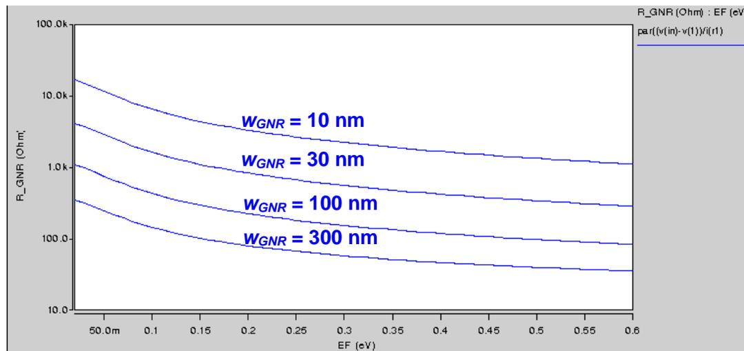
**Figure 6**  $R_{GNR}$  vs. doping level diffusion length ( $|E_F|$ ) for GNR width  $w_{GNR} = 10$  nm, 30 nm, 100 nm and 300 nm.
