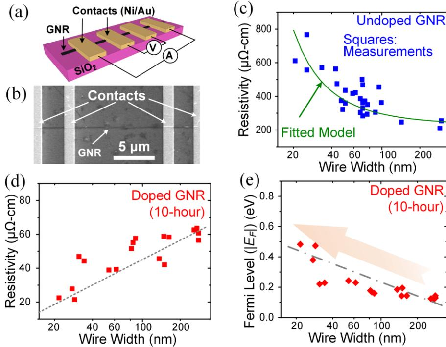
**Figure 9** (a) Schematic of 4-probe test structure. (b) Scanning electron microscope (SEM) image of test structure. (c) Fitted model with electrical measurement data for undoped GNR. (d) Measured resistivity for 10-hour doped GNR. (e) Extracted doping level for 10-hour doped GNR.
