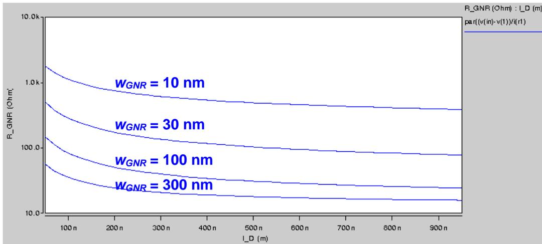
**Figure 5**  $R_{GNR}$  vs. carrier diffusion length ( $l_D$ ) for GNR width  $w_{GNR} = 10$  nm, 30 nm, 100 nm and 300 nm.
