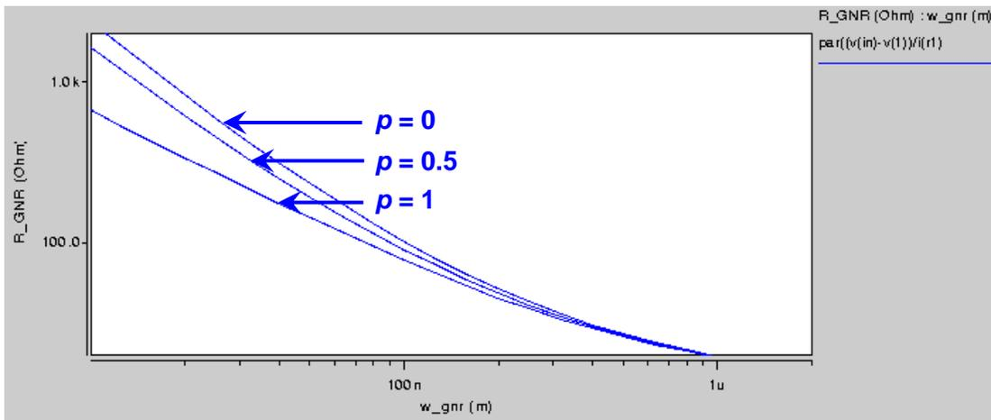
Figure 3  $R_{GNR}$  vs. GNR width  $w_{GNR}$  for edge specularity of  $p = 0, 0.5$  and  $1$ .
