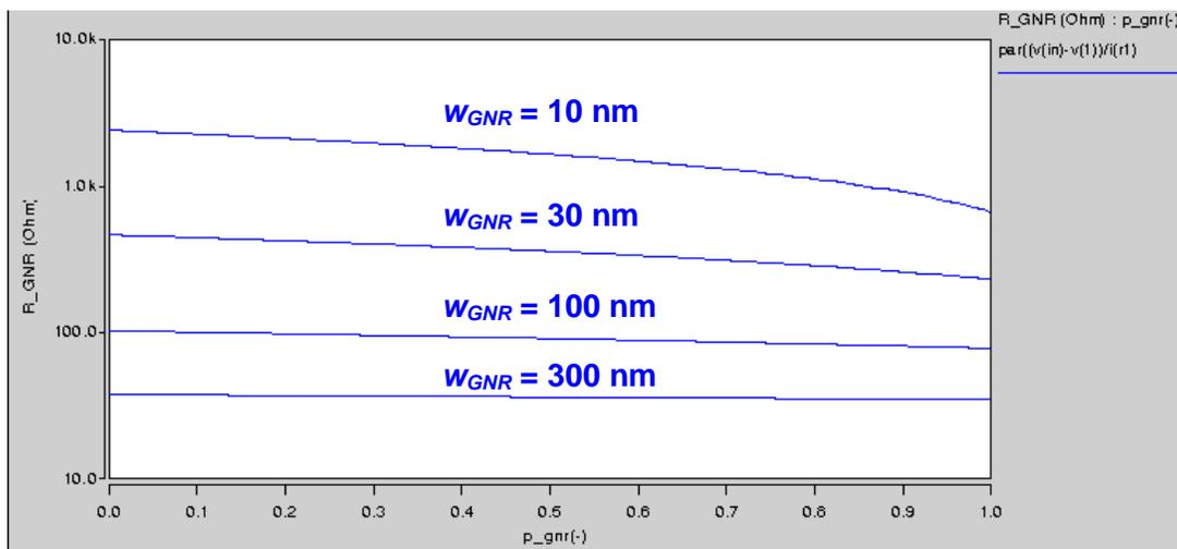
Figure 4  $R_{GNR}$  vs. edge specularity ( $p$ ) for GNR width  $w_{GNR} = 10$  nm, 30 nm, 100 nm and 300 nm.
