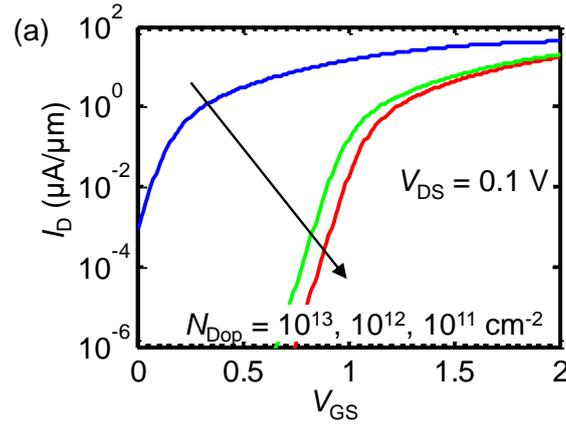
**Figure 5:** Simulated  $I_D - V_{GS}$  of a 1L single-gate MoS<sub>2</sub> n-FET with the same characteristics as in Fig. 3, but with varying doping density and  $D_{it} = 0$ . Channel doping changes the flatband (and consequently the threshold) voltage of the device.
