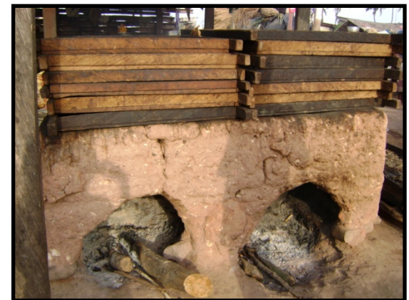
Chorkor Smoker- oven used in fish smoking
