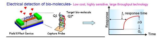
The response of a sensor is characterized in terms of its *Settling time*, *Sensitivity* and *Selectivity*. The time taken by the sensor to produce a stable signal change defines the *Settling time*. It is determined by the concentration of the analyte bio-molecules (it takes longer to detect lower concentration analyte, for obvious reasons), their diffusion coefficients in water, and their conjugation affinity (ability to bind) to the receptor molecules.
