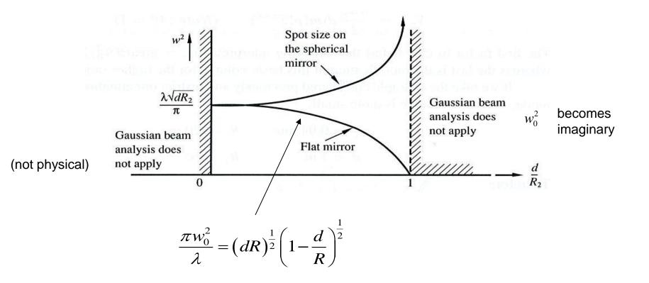
The requirement that mirrors must match the surface of the constant phase (so that a cavity mode is excited) allows one to find where the mirrors with R₁ & R₂ should be placed, in general case.
