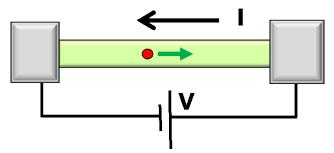
$I = G \times V$ = q × n × v × A  $\checkmark$ charge density velocity area
