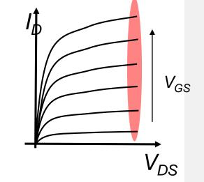
$$I_D(V_D = V_{DD}) \sim (V_G - V_{th})^{\alpha}$$
