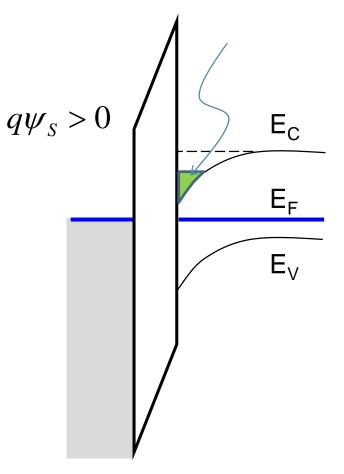
In reality, the metal and semiconductor Fermi Levels are never aligned perfectly → when you bring them together there is charge transfer from the bulk of the semiconductor to the surface so that we have alignment
