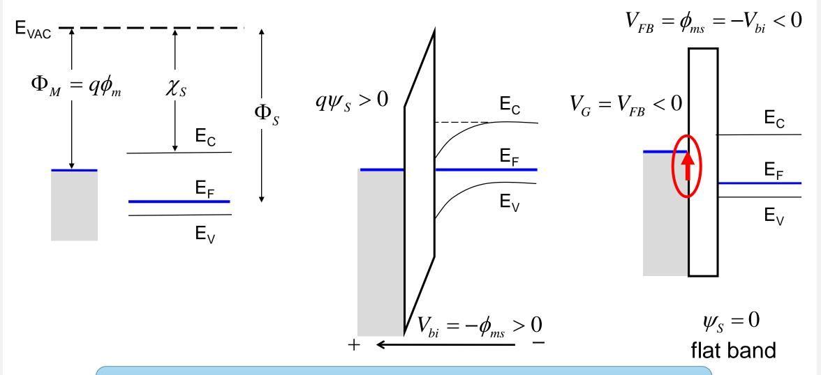
The Flatband Voltage is the voltage applied to the gate that gives zero-band bending in the MOS structure. Applying this voltage nullifies the effect of the built-in potential. This voltage needs to be incorporated into the idealized MOS analysis while calculating threshold voltage
