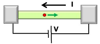
$I = G \times V$ = q × n × v × A  $\checkmark$   $\uparrow$   $\checkmark$ charge density velocity area
