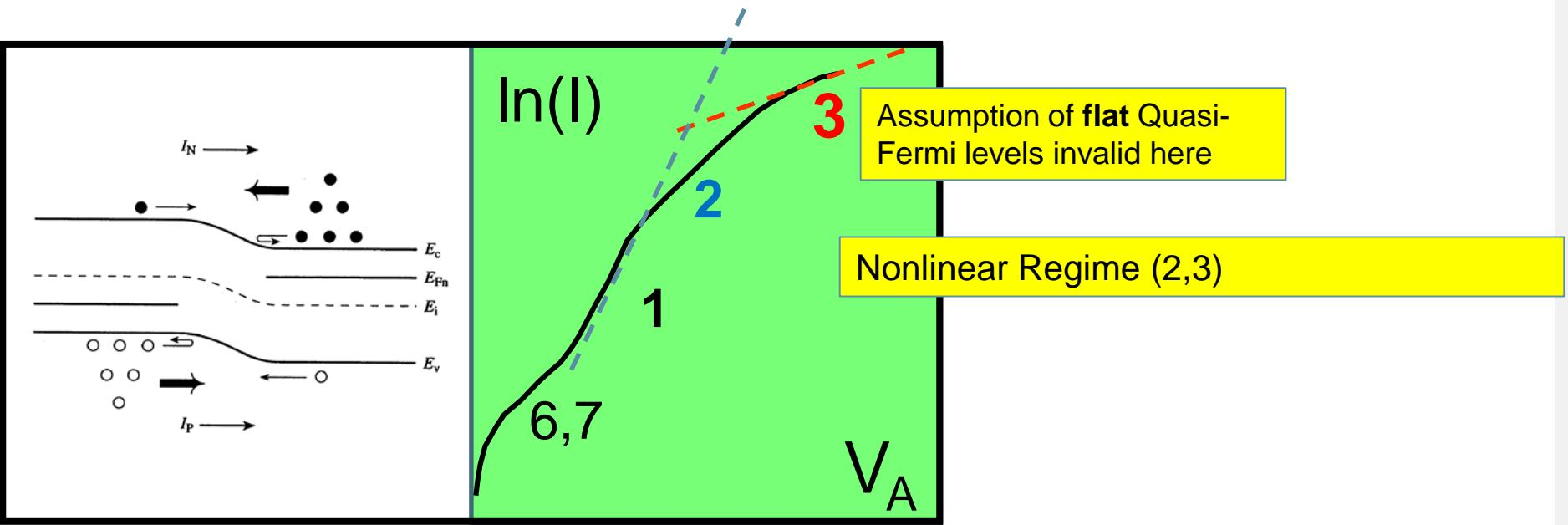
$$J_T = -q \left[ \frac{D_n}{W_p} \frac{n_i^2}{N_A} + \frac{D_p}{W_n} \frac{n_i^2}{N_D} \right] \left( e^{(qV_A - \Delta F_n - \Delta F_p)\beta} - 1 \right) = I_0 \left( e^{q(V_A - aJ_n - bJ_p)\beta} - 1 \right) = J_n + J_p$$
