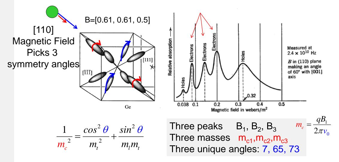
Known  $\theta$  and m<sub>c</sub> allows calculation of m<sub>t</sub> and m<sub>l</sub>.
