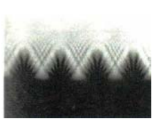
Diffraction patterns of the teeth of a saw -would be perfect geometric shadow if \lambda \rightarrow 0 (as in ray optics)
