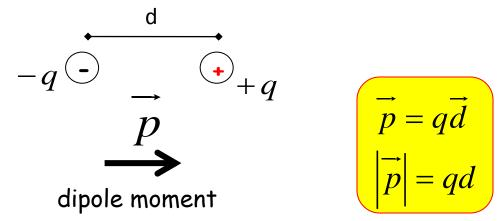
Historically the standard unit of a dipole moment was defined by two charges of opposite polarity but with equal magnitude of  $10^{-10}$  statCoulomb (also called an e.s.u. of charge - the electrostatic unit, in older literature), separated by 1 Angstrom =  $1.0 \times 10^{-8}$  cm.
