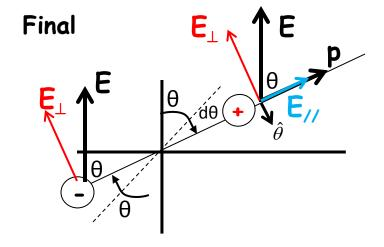
Work to rotate dipole to angle  $\theta$ :  $dW_{+} = \vec{F} \cdot d\vec{\ell} = (-qE_{\perp})\left(\frac{d}{2}d\theta\right); \quad E_{\perp} = Esin\theta$   $= -(qEsin\theta)\frac{d}{2}d\theta$   $W_{+}(\theta) = -\frac{1}{2}qdE\int_{0}^{\theta}sin\theta d\theta = \frac{1}{2}qdE[\cos\theta]\Big|_{0}^{\theta}$  $= \frac{1}{2}qdE[\cos\theta - 1]$
