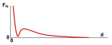
We are interested in understanding how the natural frequency of the cantilever  $\omega_0'$  could change (in the limit of infinitesimal tip vibrations) as a function of Z the cantilever sample gap. Note that  $\omega_0$  is the natural frequency in the absence of tip-sample interaction. Which of the following  $\omega_0'$  as a function of Z graphs is consistent with the  $F_{rs}$  vs d graph above? Assume that the cantilever is stiff enough for no snap-in to occur.
