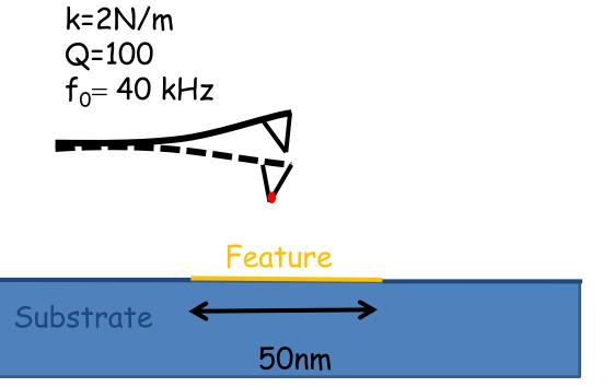
Tip-sample interaction model for substrate: Hertz Young's modulus : 150 GPA with Capillary forces
