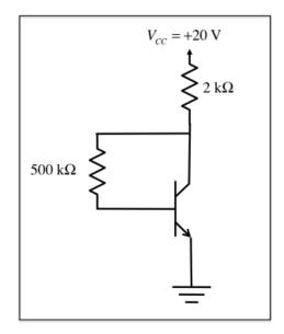
Q3. For the circuit below,  $I_{R1} = 10 I_B$ . Choose  $R_1$  so that  $I_C = 1$  mA. Assume  $\beta = 100 V_{BE} = 0.7$  V, and  $V_T = 0.026$  V. Note that you can solve this problem without knowing R<sub>2</sub>.
