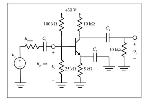
Q7. For the circuit above, what is the voltage gain,  $A_{v_i} = v_o / v_i$ ? You may assume that the capacitors are short circuits at the signal frequency. As shown in figure,  $v_i$  is to the right of C<sub>1</sub>.
