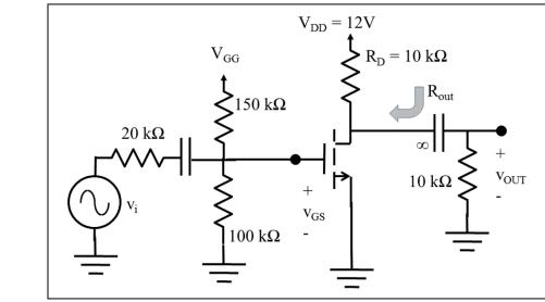
Q18 – Q19 consider the MOSFET circuit shown below. The MOSFET operates in saturation regime. At the DC bias point,  $g_m = 2 \text{ mS}$  and  $r_0 = \infty \text{ k}\Omega$ . Note that  $v_i$  is an ac small-signal source.
