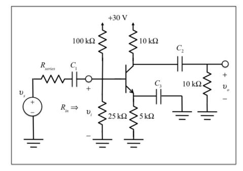
Q10. For the circuit below, what is the small signal input resistance, R<sub>in</sub>, at the indicated location?
