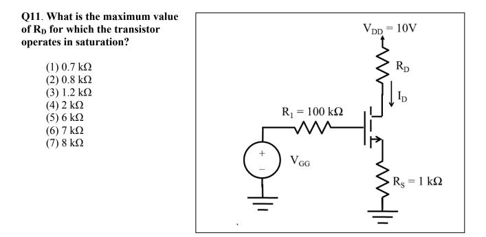
Q11 - Q12 refer to the DC MOSFET circuit shown in the figure. The MOSFET has  $V_{Tn} = 1V$  and  $\lambda = 0$ . The MOSFET operates in the saturation region and is biased at  $V_{GS} = 3V$  and drain current  $(I_D) = 1$  mA.
