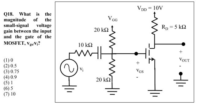
Q18 – Q19 consider the MOSFET circuit shown below. The MOSFET operates in saturation regime. At the DC bias point,  $g_m = 2 \text{ mS}$  and  $r_0 = \infty \text{ k}\Omega$ . Note that  $v_i$  is an ac small-signal source.
