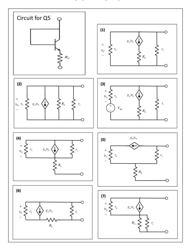
Q5. For the circuit below, select the proper small signal equivalent circuit.
