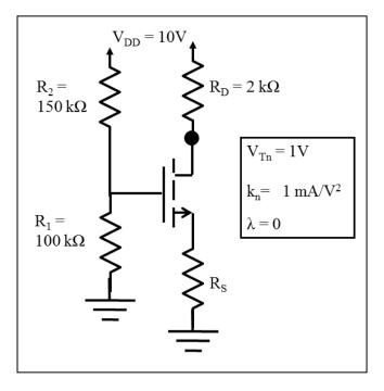
Q15 and Q16 consider an NMOS transistor with  $k_n = 1 \text{ mA/V}^2$  and  $\lambda = 0$ . The transistor is operated at  $I_D = 2 \text{ mA}$ . You are asked to find the parameters in the hybrid- $\pi$  model.
