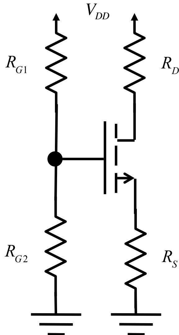
**Analysis:** Given the resistors, power supply voltage, transistor parameters, find the currents and voltages.
