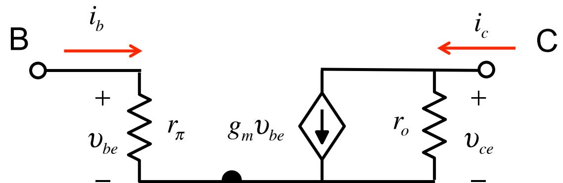
$$\boxed{\begin{aligned} g_m &= I_C / V_T \\ g_m r_\pi &= \beta \\ r_o &= V_A / I_C \end{aligned}}$$
