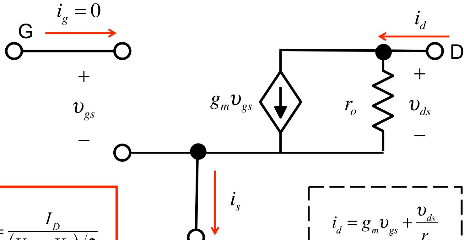
$$g_m = \frac{I_D}{(V_{GS} - V_{tn})/2}$$
