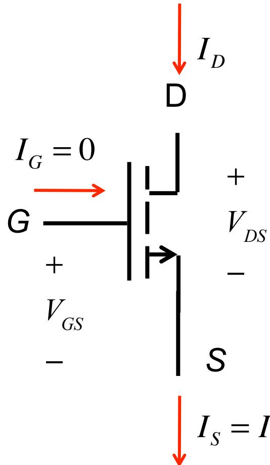
$$I_D = \frac{k_n}{2} (V_{GS} - V_{tn})^2 (1 + \lambda V_{DS})$$
