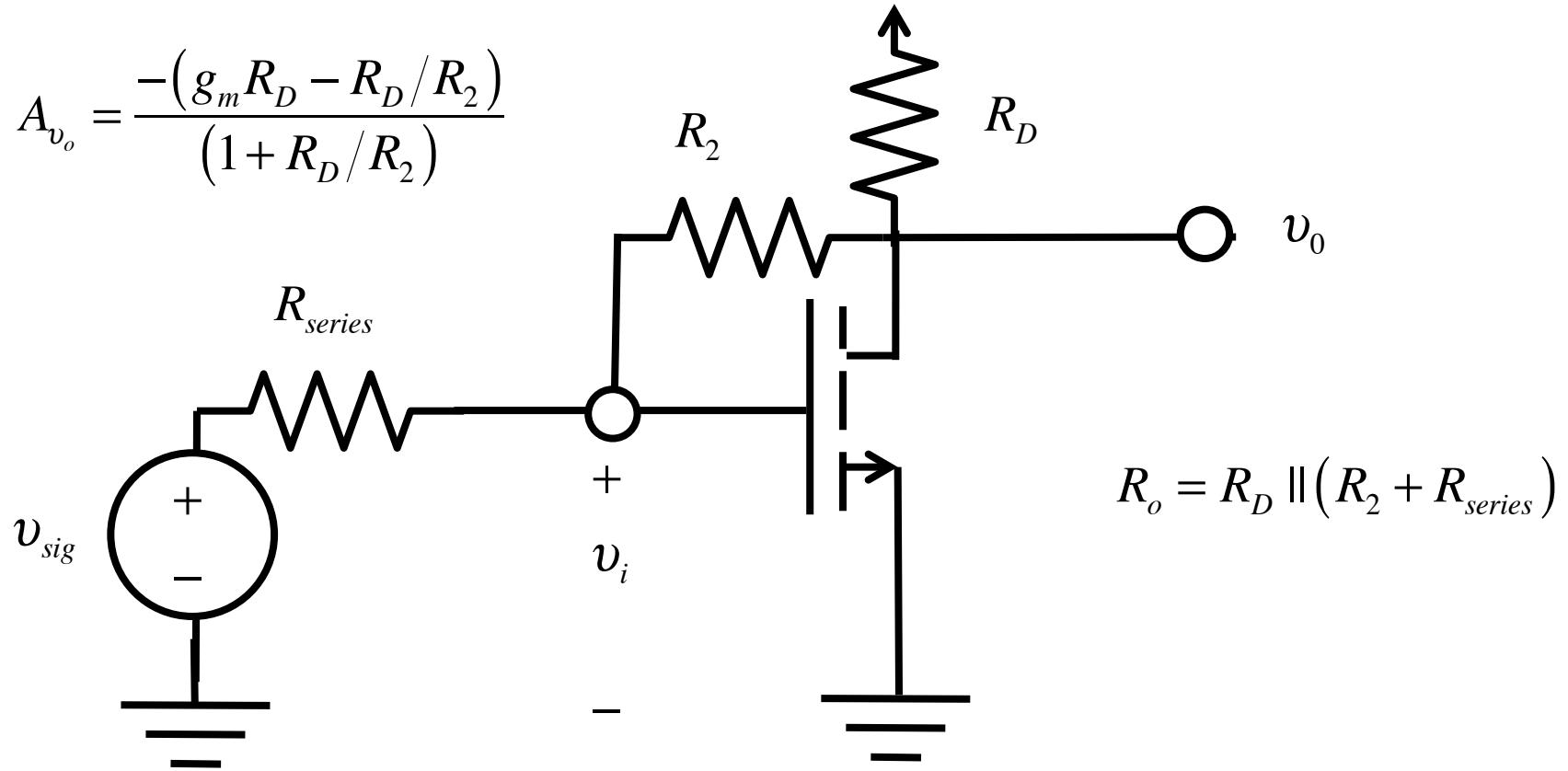
$$R_{in} = \frac{(1 + R_2/R_D)}{(1/R_D + g_m)}$$
