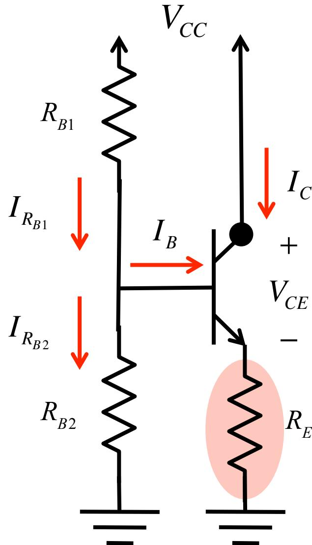
$$I_C = \frac{\beta(V_{th} - V_{BE})}{R_{th} + (\beta + 1)R_E}$$
