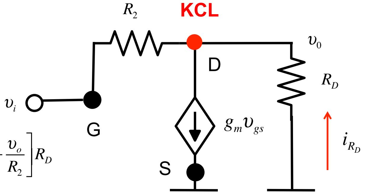
$$v_o = - \left[ (g_m - 1/R_2) v_i + \frac{v_o}{R_2} \right] R_D$$
