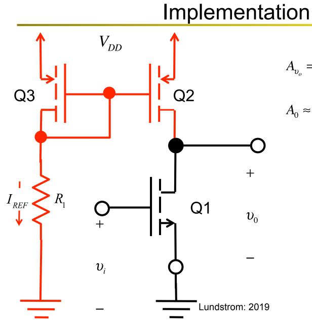
$$A_{v_o} = -g_m(r_{oN} \parallel r_{oP})$$
