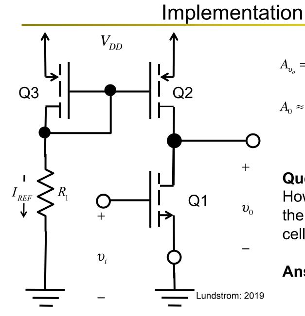
$$A_{v_o} = -g_m \left( r_{oN} \parallel r_{oP} \right)$$
