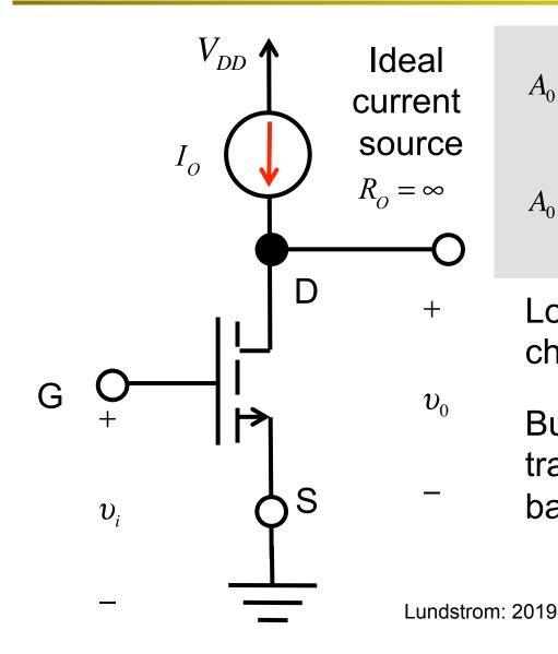
$$A_{0} = \frac{V_{A}}{(V_{GS} - V_{tn})/2} = \frac{V_{A}'L}{(V_{GS} - V_{tn})/2}$$
