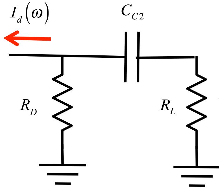
$$I_{R_L}(\omega) = I_d(\omega) \frac{R_D}{R_D + \left( R_L + \frac{1}{j\omega C_{C2}} \right)}$$
