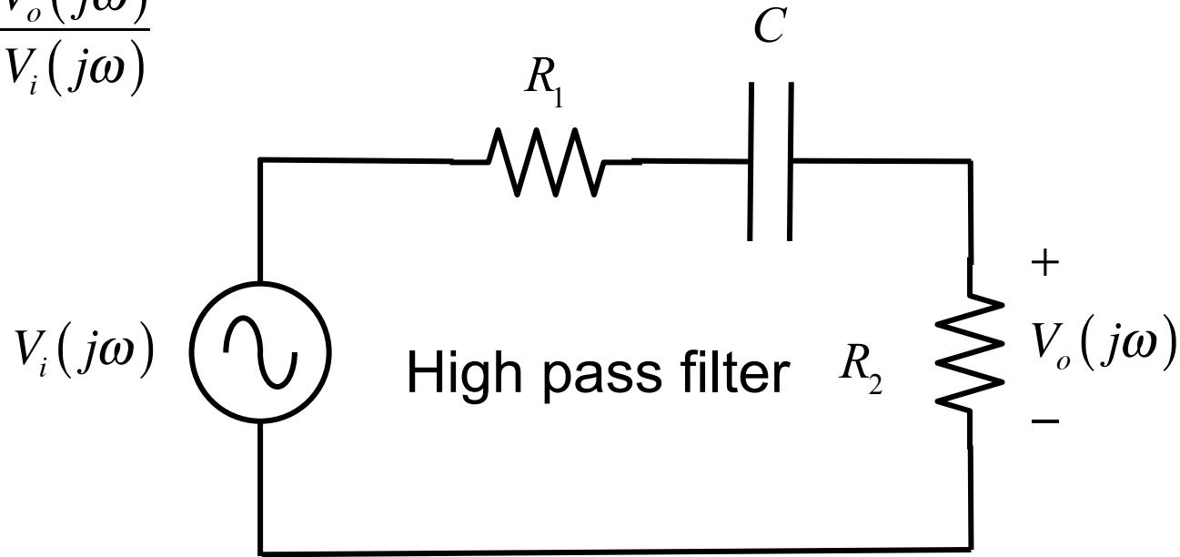
$$T(j\omega) = \frac{R_2}{R_1 + R_2 + 1/j\omega C}$$
