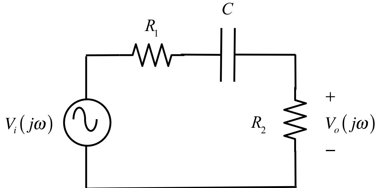
$$T(j\omega) = \frac{T_{mid}}{1 + \omega_L/j\omega}$$
