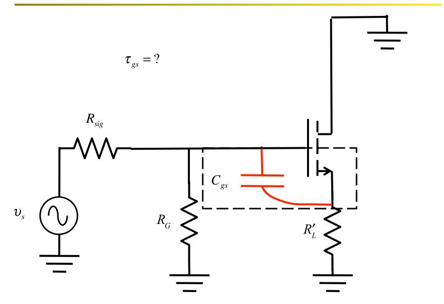
$$\tau_{gs} = R_{sig} \parallel R_G C_{in} + R'_L C_{out} \qquad \tau_{gs} = \left(R_{sig} \parallel R_G\right) C_{in} + \left[R'_L \parallel \left(1/g_m\right)\right] C_{gs}$$
