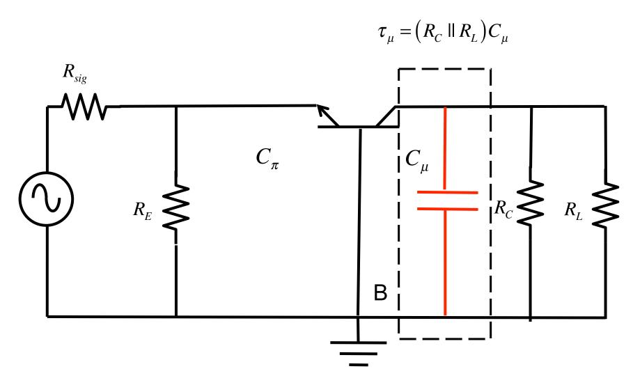
$$\begin{aligned} \tau_{\mu} &= \left( R_{C} \parallel R_{L} \right) C_{\mu} \\ \tau_{\pi} &= \left( R_{sig} \parallel R_{E} \parallel \frac{r_{\pi}}{\beta + 1} \right) C_{\pi} \\ \omega_{H} &\approx \frac{1}{\tau_{\pi} + \tau_{\mu}} \end{aligned}$$
