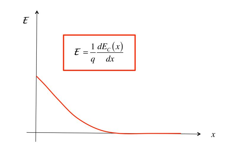
The electric field is proportional to the slope of  $E_c$
