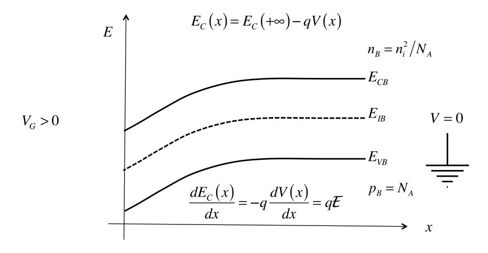
The electric field is proportional to the slope of  $E_{C_{-11}}$
