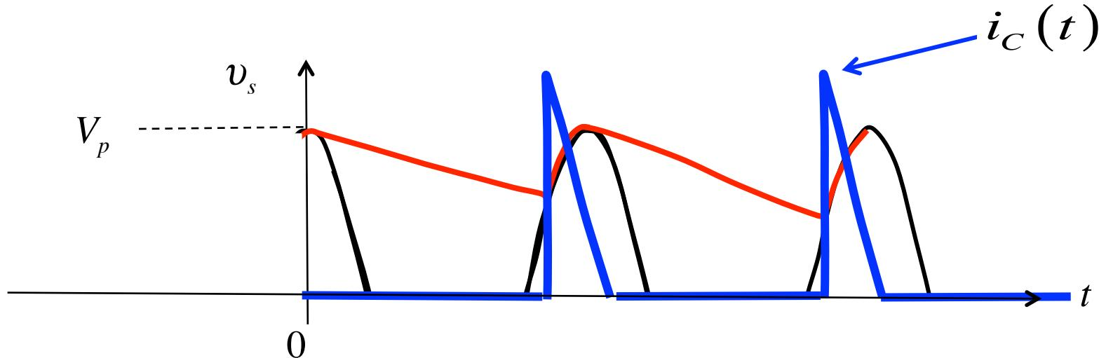
$$Q_{out} = CV_r \quad \frac{1}{2} i_C(\max) \Delta T = CV_r \quad i_C(\max) = 2 \frac{T}{\Delta T} \left( \frac{V_p}{R_L} \right) \quad \text{Large!}$$
