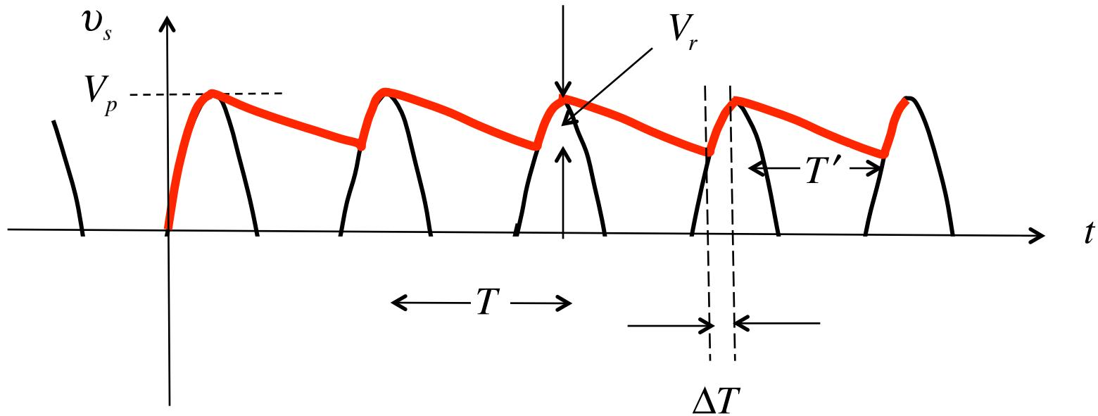
$$T' = T - \Delta T \quad \text{Good filter: } \Delta T \ll T \quad \tau = R_L C \gg T$$
