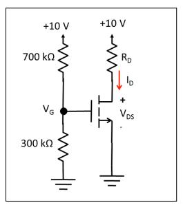
8) Consider the NMOS circuit shown in the figure to the left. Let  $V_{tn} = 0.5 \text{ V}$ ,  $k_n' = 0.1 \text{ mA/V}^2$ ,  $W_n = 4 \mu \text{m}$ ,  $L_n = 1 \mu \text{m}$  and  $\lambda = 0$ . Specify the value of the three resistors so that  $I_D = 0.2 \text{ mA}$  and  $V_{DS} = 2.5 \text{ V}$ .
