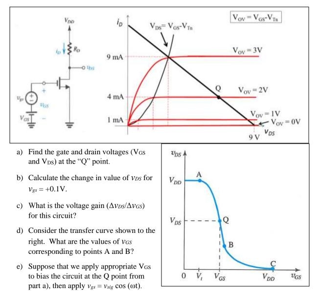
What is the maximum value of  $v_{sig}$  for which the circuit will remain in the "high gain" region (i.e. between points A and B on transfer curve?
