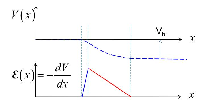
$$\mathcal{E}(x) = -\frac{dV}{dx} = \frac{1}{q} \frac{dE_c}{dx} = \frac{1}{q} \frac{dE_v}{dx} = \frac{1}{q} \frac{dE_i}{dx}$$
