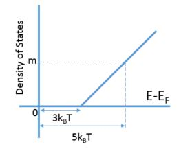
a. Using the graph, which depicts energy relative to the Fermi level  $E_F$  on the x-axis, and the density of states on the y-axis, write an expression for the density of states in terms of  $E-E_F$ .
