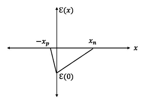
For this problem, assume that the junction is abrupt at x = 0 with a flat doping profile on each side (pdoped on the left, and n-doped on the right),  $\mathcal{E}(0) = -10$  kV/cm, n-type depletion length  $x_n = 620$ nm, and the p-type depletion length  $x_p = 100$  nm.
