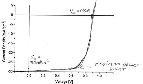
c. Assuming that the cell is illuminated by the AM1.5 solar spectrum ( $P_{in}=100~{\rm mW/cm^2}$ ), calculate the maximum power conversion efficiency.
