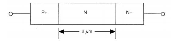
Also assume that  $V_{bi}=1.1$  V,  $K_s$ =12,  $J_o=0.14$  nA/cm²,  $\tau=1~\mu s$ , and that the capacitance as a function of voltage is measured as below:
