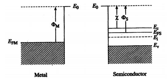
a. (10 pts) Draw the equilibrium band diagram for an ideal metal-semiconductor (MS) structure formed from the pictured components with the indicated parameter values.
