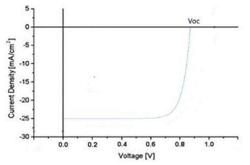
c. Assuming that the cell is illuminated by the AM1.5 solar spectrum ( $P_{in} = 100 \text{ mW/cm}^2$ ), calculate the maximum power conversion efficiency. Also, calculate the efficiency if the doping of both sides of the solar cell is increased by a factor of ten, while the short circuit current remains the same, assuming the ideal diode dark current holds, and the mobility is unchanged.
