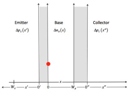
3c) The concentration of excess minority carrier electrons at the beginning of the base,  $\Delta n_B(0)$ , is indicated by the filled circle on the figure above. Determine numerical values of the excess minority electron density at the two ends of the base,  $\Delta n_B(0)$  and  $\Delta n_B(W_B)$  and sketch  $\Delta n_B(x)$  within the base.
