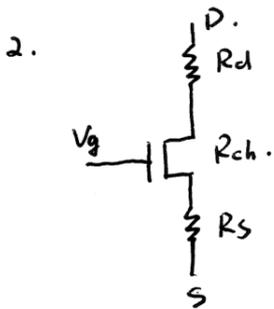
the effective  $V_{gs} = V_{gs} - I_d \cdot R_s$ .
