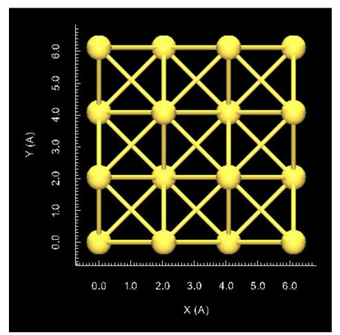
1.a) (001) surface of FCC gold is the x-y plane of the lattice.
