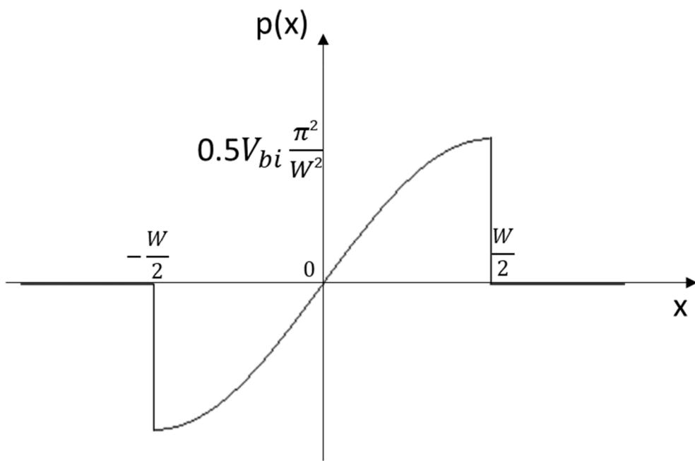
d)  $N_D - N_A = p(x)/q = 1/q \frac{dE}{dx} = 0.5 \frac{V_{bi}}{K_s \epsilon_o} \frac{\pi^2}{W^2} \sin(\frac{\pi x}{W})$
