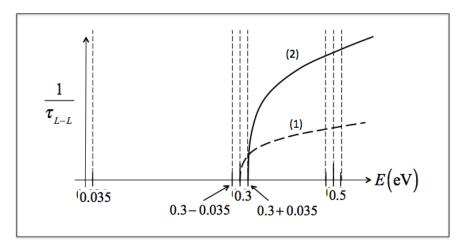
An electron at the bottom of an L-valley can absorb a phonon and scatter to another L-valley, but an electron near the bottom of an L-valley cannot scatter to another L-valley by emission, because there are no L-valley states available at that energy.
