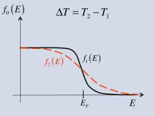
$|f_1 - f_2| > 0$  so current flows, but the sign depends on whether the states are located above or below  $E_F$  (n-type or p-type).
