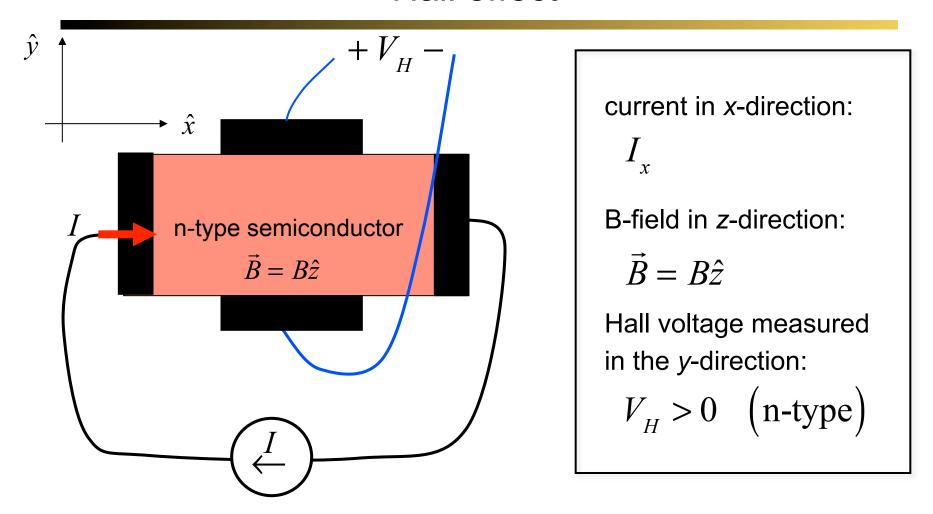
The Hall effect was discovered by Edwin Hall in 1879 and is widely used to characterize electronic materials. It also finds use magnetic field sensors.
