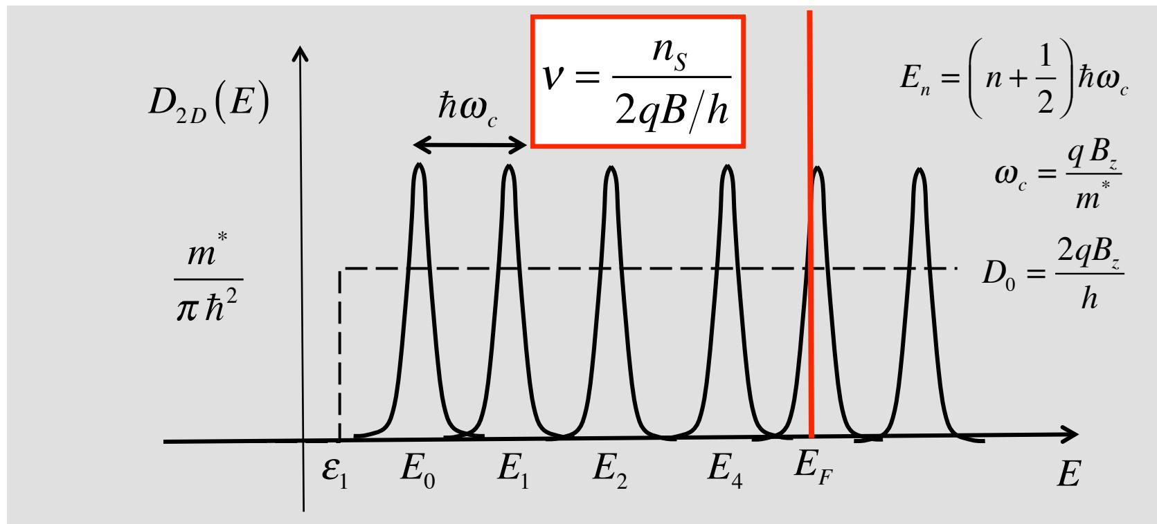
For a given sheet carrier density,  $n_s$ , some (fractional) number of LL's are occupied.
