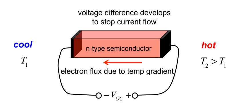
Temperature gradients give rise to an open circuit voltage, which is known as the Seebeck effect. We expect a **positive** voltage for an n-type semiconductor (and **negative** voltage for a p-type semiconductor.)
