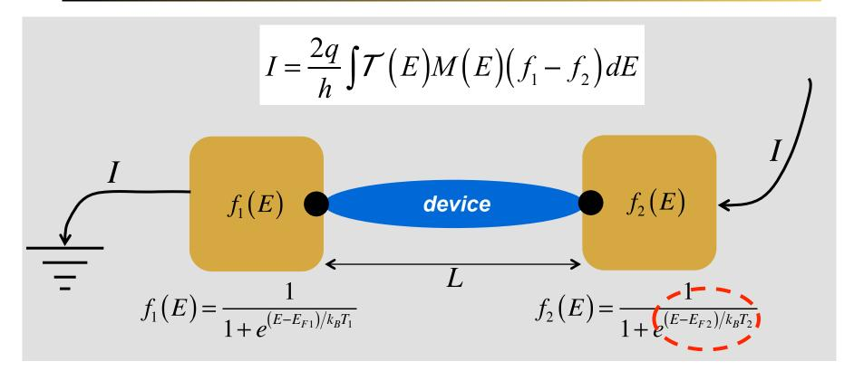
**Driving "forces" for current flow:** Differences in Fermi level and differences in temperature.
