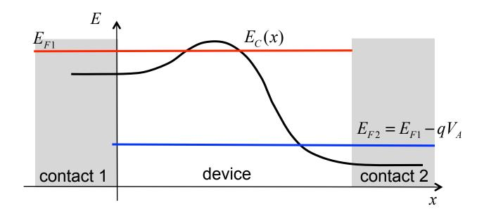
Inside the devices, some states are occupied according to the Fermi level of the first contact and some according to the Fermi level of the second contact.
