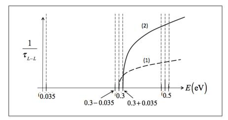
An electron at the bottom of an L-valley can absorb a phonon and scatter to another L-valley, but an electron near the bottom of an L-valley cannot scatter to another L-valley by emission, because there are no L-valley states available at that energy.
