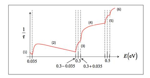
The scattering rate is the sum of 6 different processes; the last five of these have thresholds for their onset.
