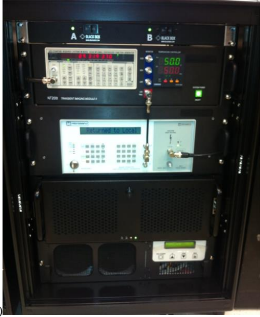
Figure 1: Picture of the system a) microscope setup and b) signal inter-lock and processing unit
