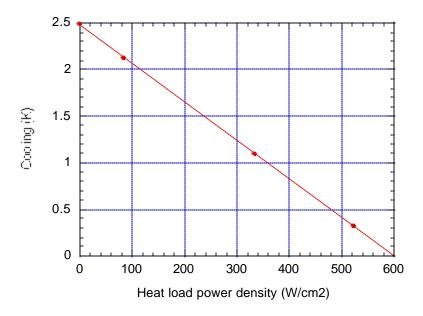
Fig. 4 Measured cooling power density for 40  $\times$  40  $\mu m^2$  SiGe/Si cooler at room temperature.
