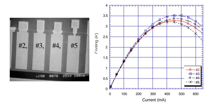
Fig. 1 (a) Devices with an area of 6400  $\mu$ m<sup>2</sup> and with different side pad widths. (b) Measured cooling on top of the device versus current.
