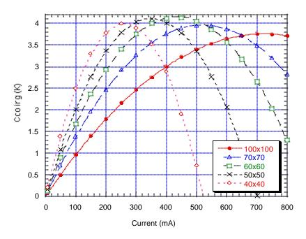
Fig. 3 Cooling measured on top of the device versus current for  $40 \times 40 \,\mu\text{m}^2$ ,  $50 \times 50 \,\mu\text{m}^2$ ,  $60 \times 60 \,\mu\text{m}^2$ ,  $70 \times 70 \,\mu\text{m}^2$  and  $100 \times 100 \,\mu\text{m}^2$  SiGe/Si coolers.
