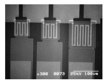
Fig. 2 Processed SiGe/Si coolers with integrated thin film metal wire resisters.
