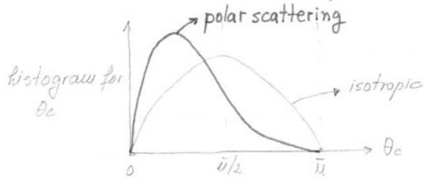
For polar optical phonon scattering and for ionized impurity scattering, where small angle scattering is preferred the weight will shift towards  $\theta_c = 0$ .
