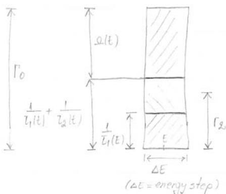
To be able to use random numbers uniformly distributed between 0 and 1, all cumulative rates are renormalized with  $\Gamma_0$ . Then, a particular scattering mechanism is selected when:
