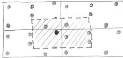
For a given carrier, a second volume is defined that is centered around the carrier when the interparticle forces are being calculated. Then:
