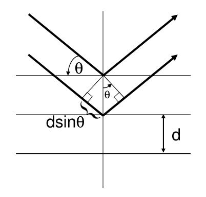
The difference in the paths traversed by the two beams shown in the figure is:
