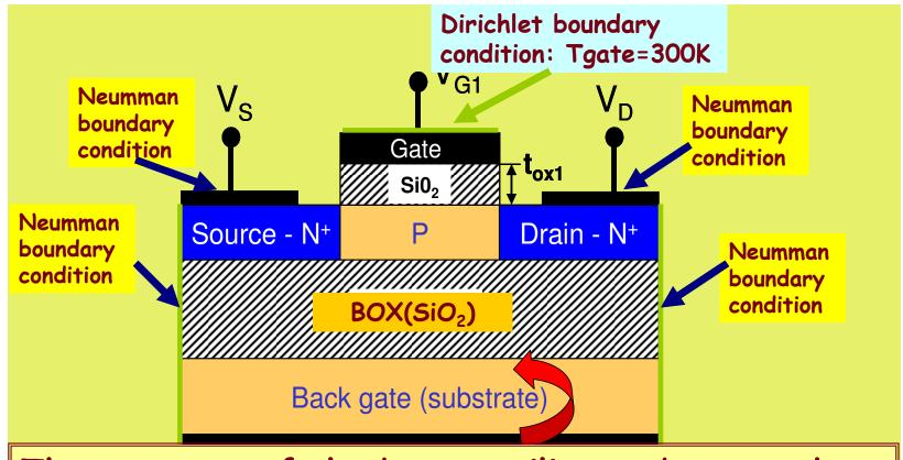
The presence of the bottom silicon substrate does not affect either the electrical or the thermal characteristics of the structure being considered.
