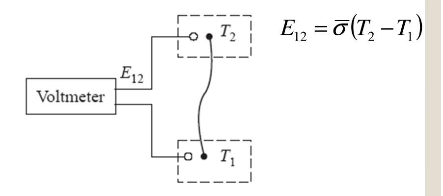
where  $\overline{\sigma}$  is the average Seebeck coefficient for the wire material over the temperature range  $T_1 \leq T \leq T_2$ .
