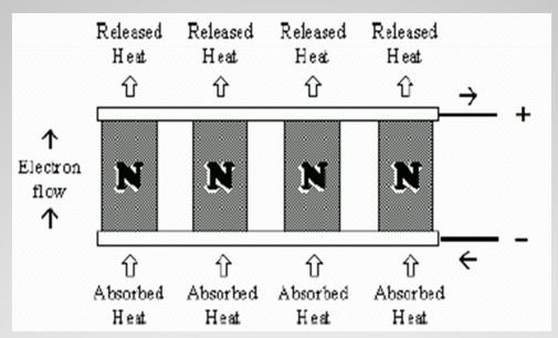
The TE components can be put in series but the heat transport abilities are diminished because the interconnectings between the semiconductor creates thermal shorting.
