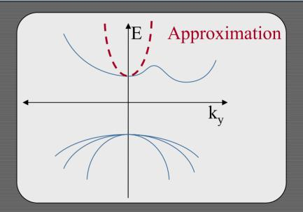
For nano-tubes we can derive a similar parabolic expression via a Taylor series expansion that approximates the subbands near the conduction valleys
