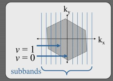
• This is how constraints along a given dimension result in subbands. *Note:* For carbon nano-tubes with a very large circumference, the number of subbands in the Brillouin Zone can be so great that its behavior is indistinguishable from that of graphite
