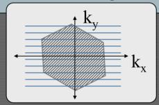
• A nano-tube will only conduct if one of its subbands pass through the six corners of the Brillouin Zone. So condition for conduction is
