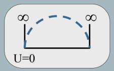
• GaAs sandwiched between two blocks of AlAs provides a real world example of this...
