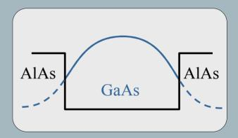
Of course, the "infinite" barrier is not really infinite and there is some leakage of the wavefunction (this is shown above)
