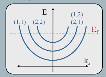
• As a conductor increases in size the subbands get closer together, with the Fermi energy remaining unchanged this means that the resistance goes down! (More modes lie below the Fermi energy)
