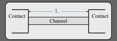
• The minimum resistance comes from the contact resistance. The smaller the device the more important this contact resistance. One might assume that this resistance may be eliminated by improving the contacts; this simply is not true. There is a minimum contact resistance.
