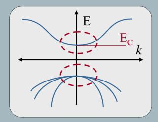
• We are largely interested in the areas circled above because they determine the conduction and optical properties of a material. To simplify matters we create a parabolic model of the curvature in these areas
