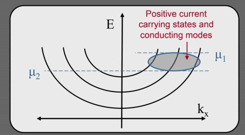
Given a quantum wire of length L, how do we calculate the current carried? • First, the number of electrons available for conduction is given by
